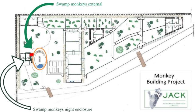
Located at the middle of the J.A.C.K. Center's monkey project, the outside enclosure is a 16 m long, 12 m wide and 8 m high structure. Meshed and wooded, it features platforms, galvanized bars and feeders and drinkers. The entire enclosure is built around a large fig tree on a former termite mound. A tunnel links the external enclosure to the night rooms. For safety reasons, the monkeys will be brought in every evening just like the others.
