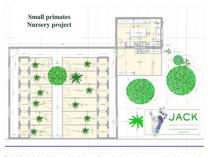
The building includes a kitchen, a mini-clinic, a small room for the vet or keeper to spend the night in case of emergency, and 12 night lodges attached to 12 eight-meter-high day enclosures with vegetation so that the individuals can move around by jumping in a natural environment.
